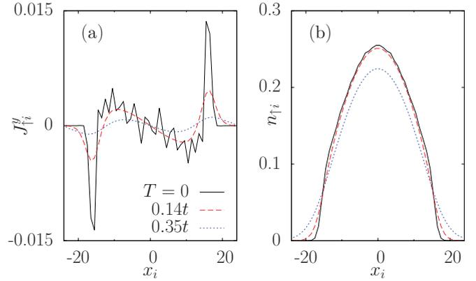
FIG. 4. (Color online) (a) The strength of the  $\uparrow$  mass current  $J_{\uparrow i}^y$  (in units of  $t$ ), and (b) the filling of  $\uparrow$  fermions  $n_{\uparrow i}$  at finite  $T$  as a function of  $x_i$ , when  $y_i = 0$ . Here, the system is noninteracting and SOC is symmetric with  $\alpha = \beta = \pi/4$ , and we set  $T$  to 0 (solid black)  $0.14t$  (dashed red), and  $0.35t$  (dotted blue). Coarse-grained data are a finite-size lattice effect.
